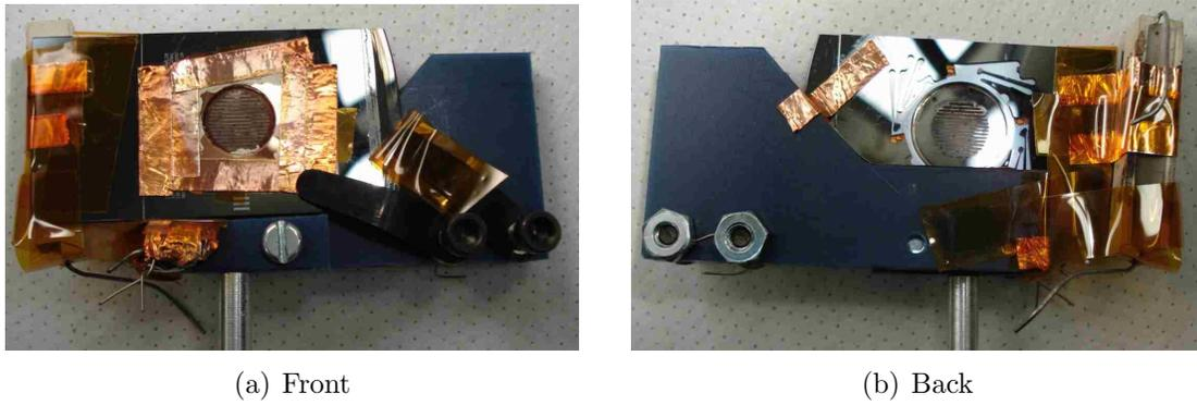
Figure 6-1: The thruster (without the emitters) mounted in its polyethylene holder. A heating resistor is attached to the thruster in these pictures
