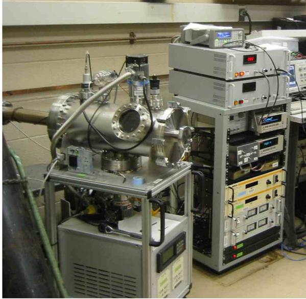
Figure 6-4: The vacuum chamber (left) and power supplies (right) for the experiment
