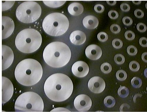
Figure 5-6: The test device that was used to evaluate the electrical properties of the Insulating Substrate insulation method. Trenches 1 mm, 2 mm and 4 mm thick were cut around 2 mm diameter contacts
